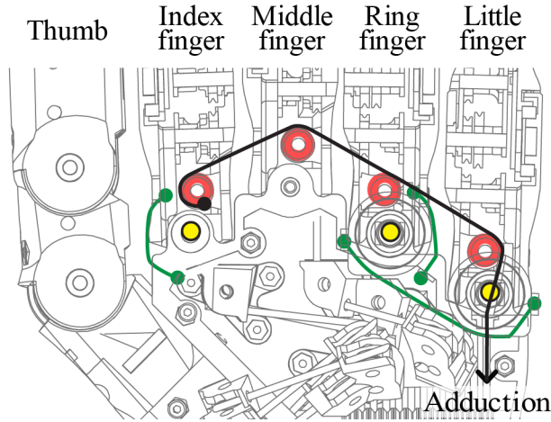
Figure 4.18: Saggital section view of the palm shows abduction and adduction mechanism.
