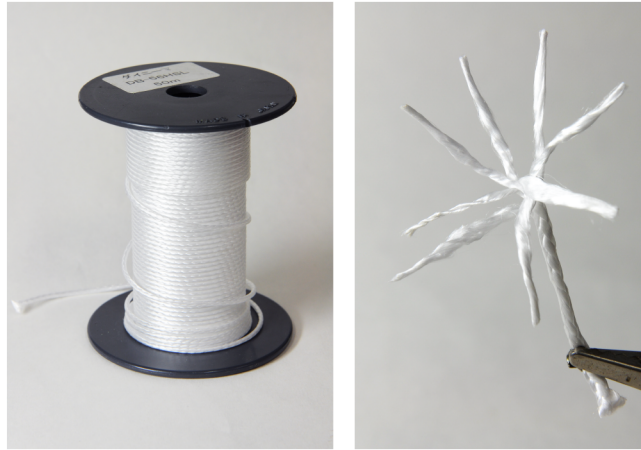
Figure 3.10: DB-56HSL 1.5 mm Dyneema™ tendon from Humilon Company.
